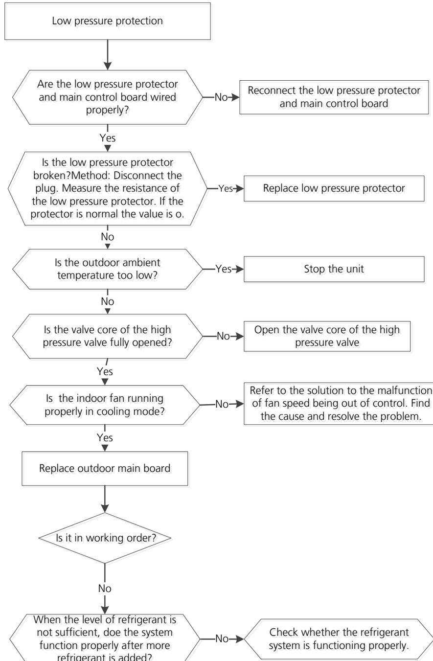
**Note:** For certain models, outdoor PCB could not be removed separately. In this case, the outdoor electric control box should be replaced as a whole.
