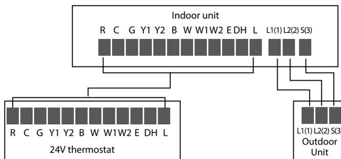
NOTE: The wiring method of the thermostat and the internal machine refers to the wiring of the non-communication scheme.
