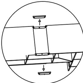
Remove knockouts as shown in the figure.
