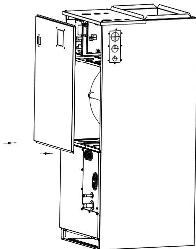
14. Reinstall the filter and filter cover plate.
