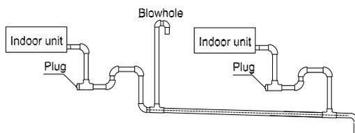
9. The end of drainage pipe shall not contact with ground directly.
