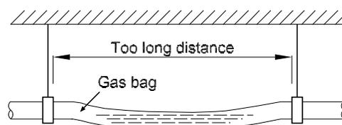
5. The horizontal pipe layout should avoid converse flow or bad flow
