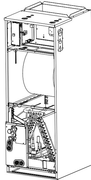
4. Unplug temperature sensors T1,T2 from the control board.
