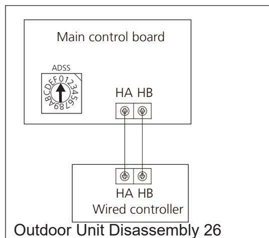
For some models: The wired controller connects to terminal board, terminal board connects to main control board.
