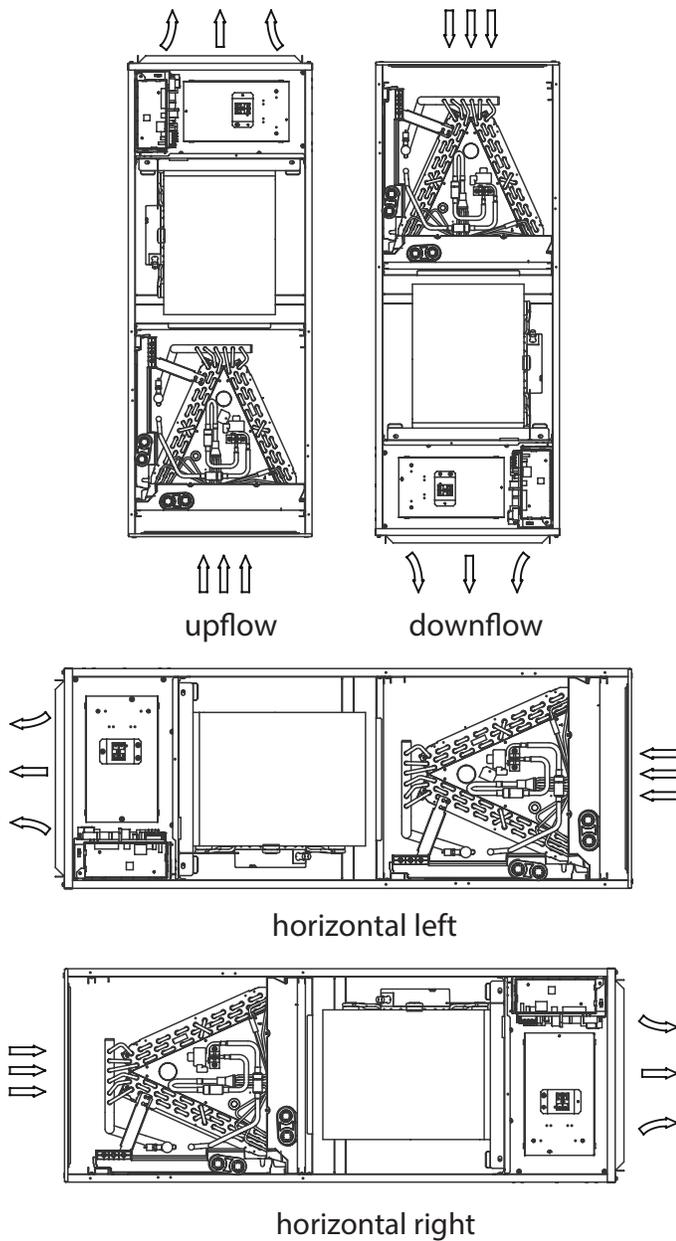
For the Horizontal left installation and vertical down installation, the direction of the evaporator should be changed and the drain pan should be removed first. Please do it according to the following steps:
