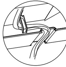
Hook the wire into the buckle and go down from the wire slot.
