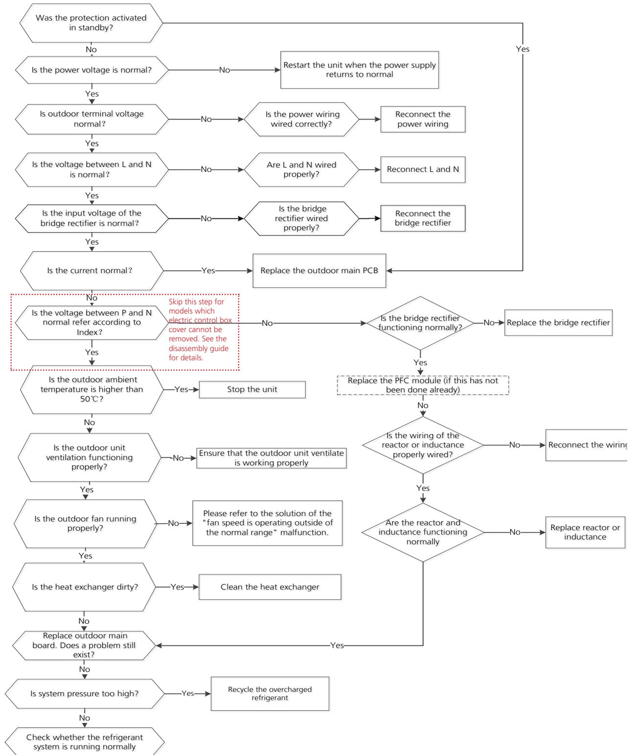
**Note:** For certain models, outdoor PCB could not be removed separately. In this case, the outdoor electric control box should be replaced as a whole.
