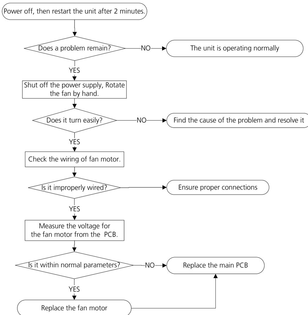
**Note:** For certain models, outdoor PCB could not be removed separately. In this case, the outdoor electric control box should be replaced as a whole.
