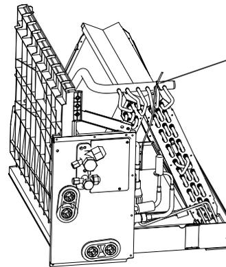
Use cable ties to fix the room temperature sensor as shown in the figure.
