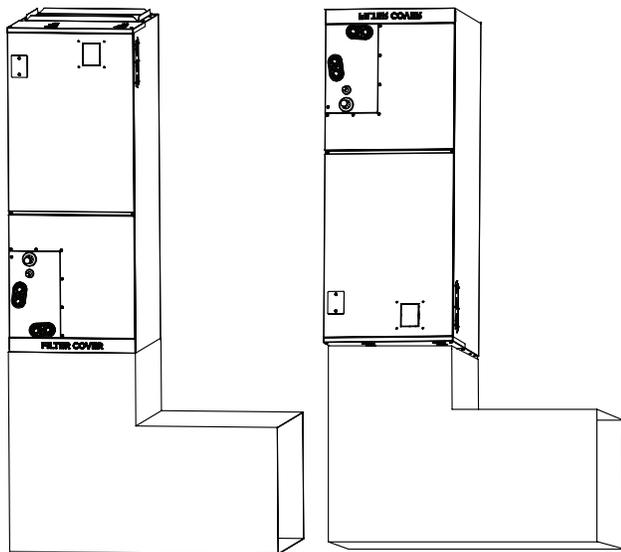
When installed vertically (upward or downward), the lower end of the air outlet needs to be connected to the L-shaped metal air duct and fastened by screws.
